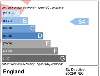
The environmental impact rating is a measure of a home's impact on the environment in terms of carbon dioxide  $(CO_2)$  emissions. The higher the rating the less impact it has on the environment.
